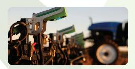
Our technology allows for two additional operating modes: dual spraying and cover mode. In dual spraying, you can apply low application rates (like 30 l/ha) full width and higher rates (like 100 l/ha) with just one spray line.
