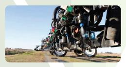
Cover mode feature allows you to use while during weed and grass spraying. Your sprayer acts as a normal sprayer but with pulse width modulation (PW) to maintain the set spray rate independent to the operation speed and book movement.
